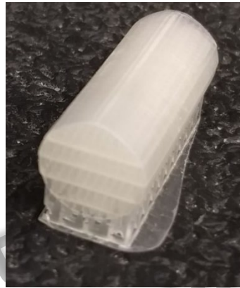
3D printed bioreactor (~ 2.5 cm 3 )
